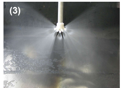
(3) Adaptor with 7 flat spray nozzles mounted
