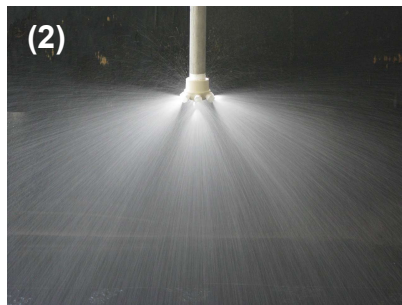
(2) Adaptor with 7 full cone spray nozzles mounted
