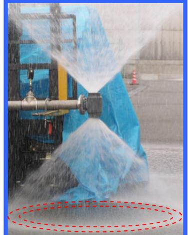
With 2 orifices, the flow normally sent through 1 orifice is halved, yielding smaller droplets. Best for applications with contact / reactions.
