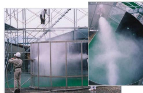
Actual simulation in a model cooling tower
