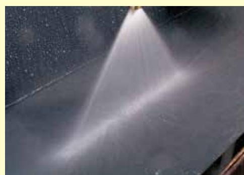
The increased thickness of the flat spray from this nozzle allows for more effective cooling in the space between rolls.
