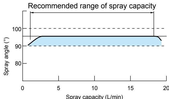
The variation in spray angle is minimized despite the large modulation of spray capacities.
